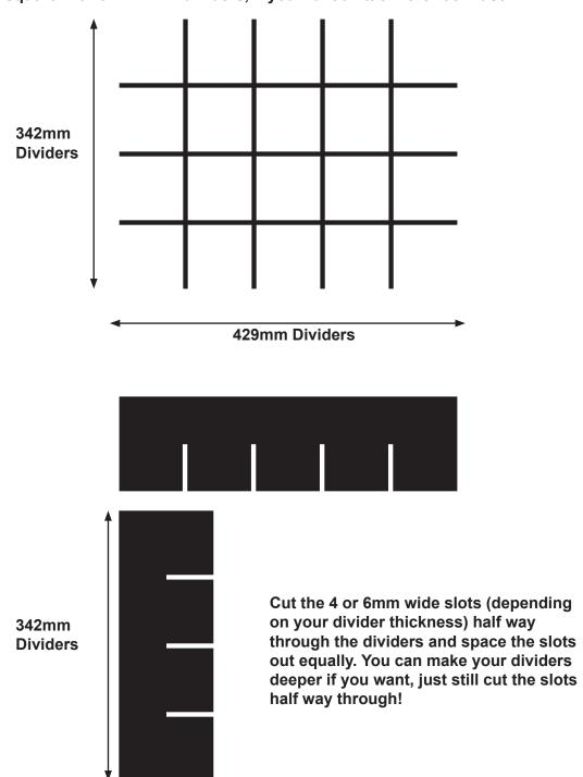
I was thinking of PVA wood glue and some 25mm Panel pins for the construction of the 10mm box, then the dividers could just be glued in place once you've made them fit.
